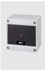
RCI WRR-22 2-Channel receiver 433MHz 2-channel Wiegand output long-range receiver. Read range up to 100 ft (30.5m) 3.4" W x 6.3" H x 2.3" D (86.4 x 160 x 58.4 mm)
