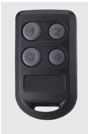
RCI WRT-4+H 4 button transmitter Button press – 433 MHz rolling code and encrypted. Presentation – 125 kHz Proximity Range: Button press Up to 200 feet (61 m), Presentation Up to 3.5 inches (88 mm) 1.45" W x 2.5" H x 0.56" D (37 x 63.5 x 14.2 mm)
