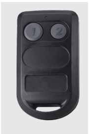
RCI WRT-2+D2 2 button transmitter Button press – 433 MHz rolling code and encrypted. Presentation – 13.56 MHz MIFARE DESFire EV2 Range: Button press Up to 200 feet (61 m), Presentation Up to 3.5 inches (88 mm) 1.45" W x 2.5" H x 0.56" D (37 x 63.5 x 14.2 mm)
