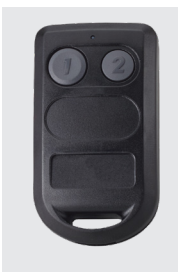
RCI WRT-2+H 2 button transmitter Button press – 433 MHz rolling code and encrypted. Presentation – 125 kHz proximity Range: Button press Up to 200 feet (61 m), Presentation Up to 3.5 inches (88 mm) 1.45" W x 2.5" H x 0.56" D (37 x 63.5 x 14.2 mm)
