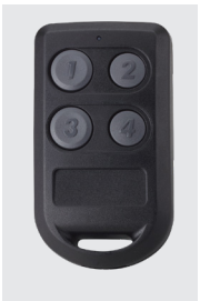
RCI WRT-4+D2 4 button transmitter Button press – 433 MHz rolling code and encrypted. Presentation – 13.56 MHz MIFARE DESFire EV2 Range: Button press Up to 200 feet (61 m), Presentation Up to 3.5 inches (88 mm) 1.45" W x 2.5" H x 0.56" D (37 x 63.5 x 14.2 mm)
