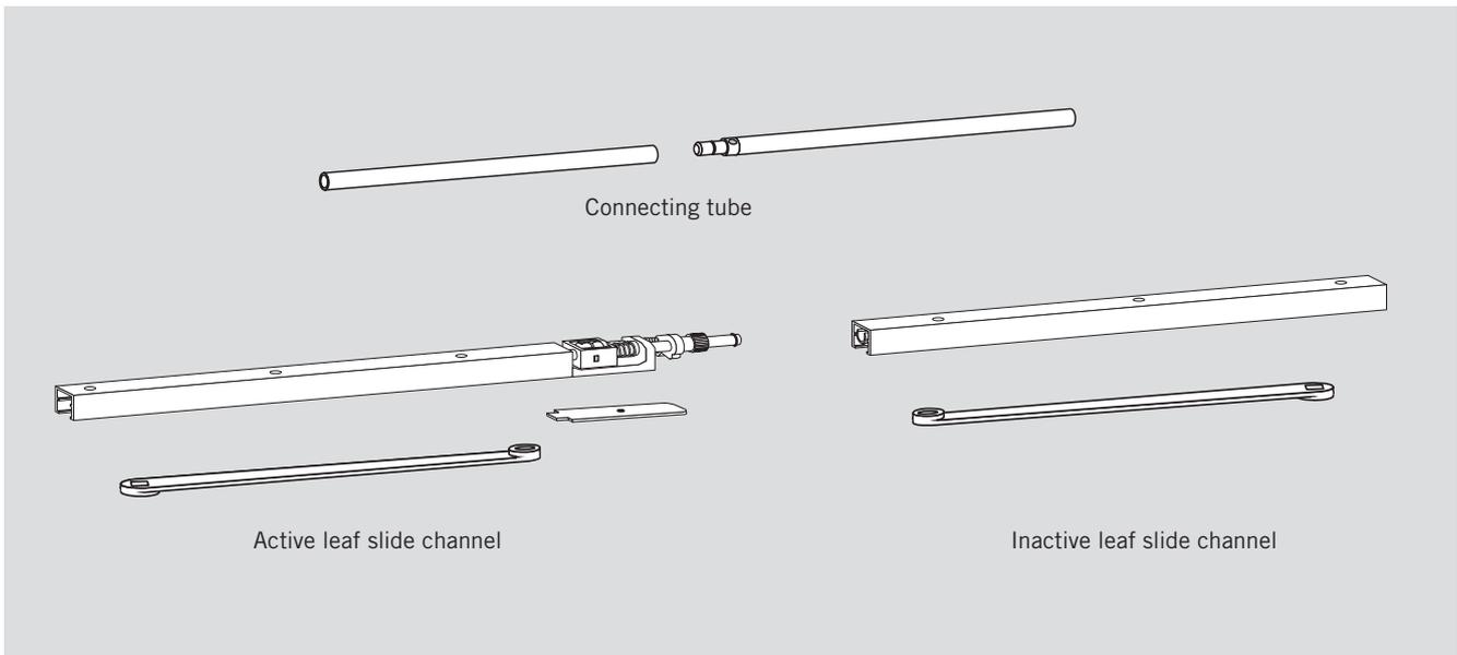
A slide channel door co-ordinator encompasses an active leaf and an inactive leaf slide channel with cushioned limit stay, a connecting tube, a cover for the co-ordinator mechanism on the active leaf slide channel, and two arms.
