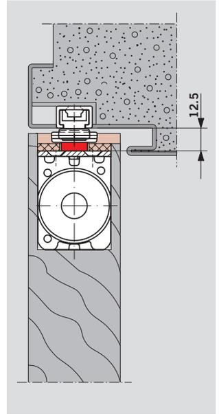
Tubular steel frame door, flush-closing, clearance 12 mm, with ITS 96/ITS 96 FL EN 3-6 and slide channel G 96 N20 K12.
