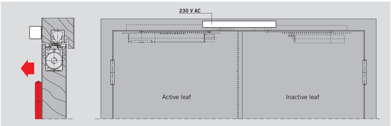
RMZ frame-mounted smoke detector on the pull side connected to an ITS 96 FL GSR.
