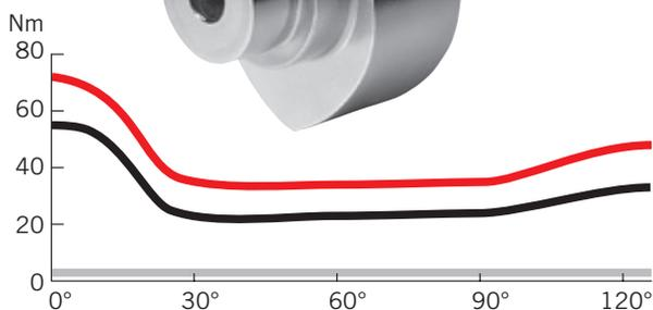
Force profile of an ITS 96 cam-action door closer (Size EN 3 – 6, max. closing strength setting)
