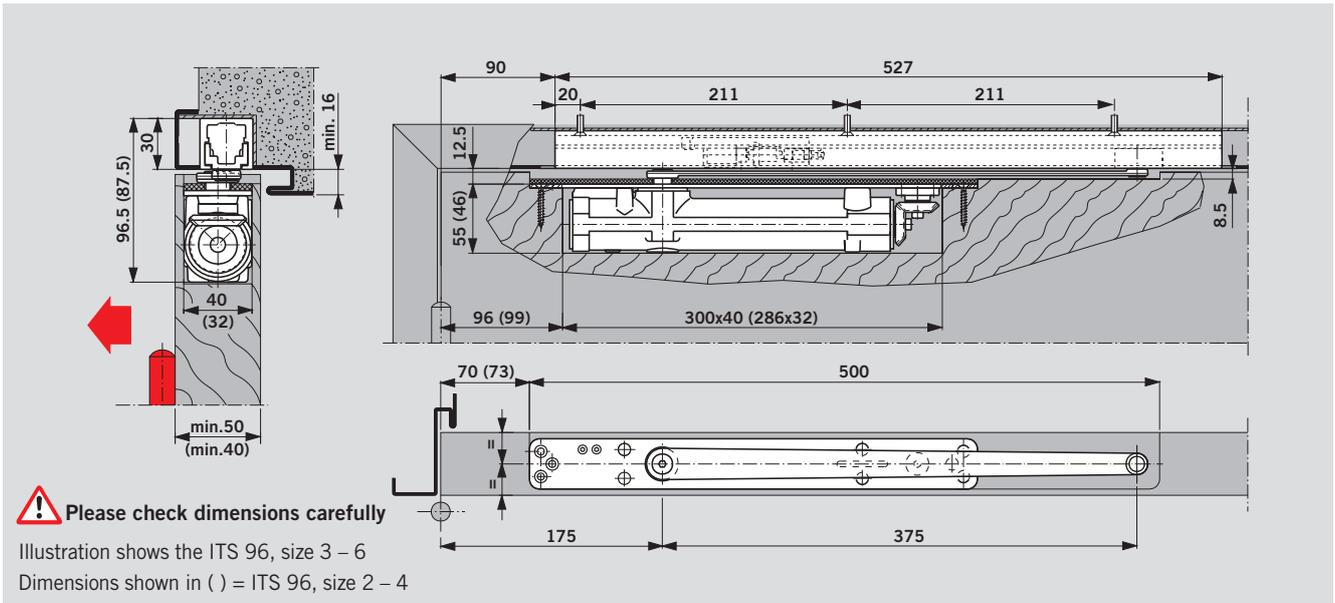
ITS 96 door closer with DORMA G 96 EMF slide channel assembly in a **timber door**.
