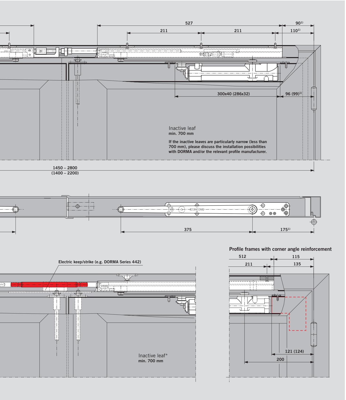
**F** When installed in fire and smoke check doors, ensure that the DORMA MK 397 carry bar is also fitted.
