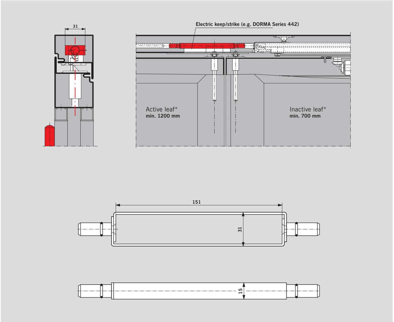
Connecting frame for G 96 GSR door co-ordinator for use on doors with electric keep/strike or overhead electro-mechanical locking device
