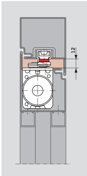
Aluminium tubular frame door, flush-closing, clearance 16 mm, with ITS 96/ITS 96 FL EN 3-6, 4 mm extended spindle and slide channel G 96 N20 K12.
