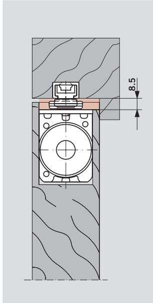
Timber door with steel frame, flush closing, clearance 12.5 mm, with ITS 96/ITS 96 FL EN 3-6, 4 mm extended spindle and slide channel G 96 N20 K8.
