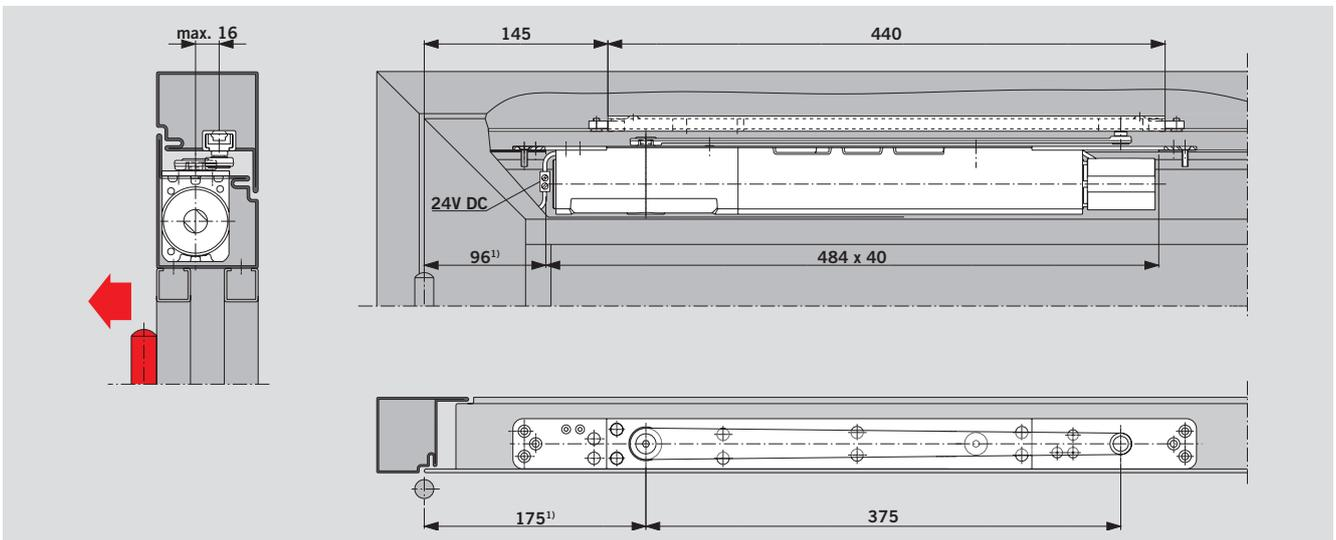
ITS 96 FL door closer with DORMA G 96 N20 slide channel in an **aluminium framed door**. Example: Anticlockwise-closing (ISO 6) door; mirror image applies to clockwise-closing (ISO 5) doors. <sup>1)</sup> Add 25 mm for aluminium profile frames with corner-angle reinforcement.
