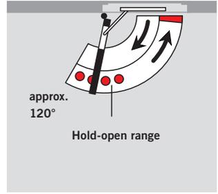
The RF hold-open unit enables doors to be securely held without any fall-back at precisely the required position up to an opening angle of approx. 120°.
