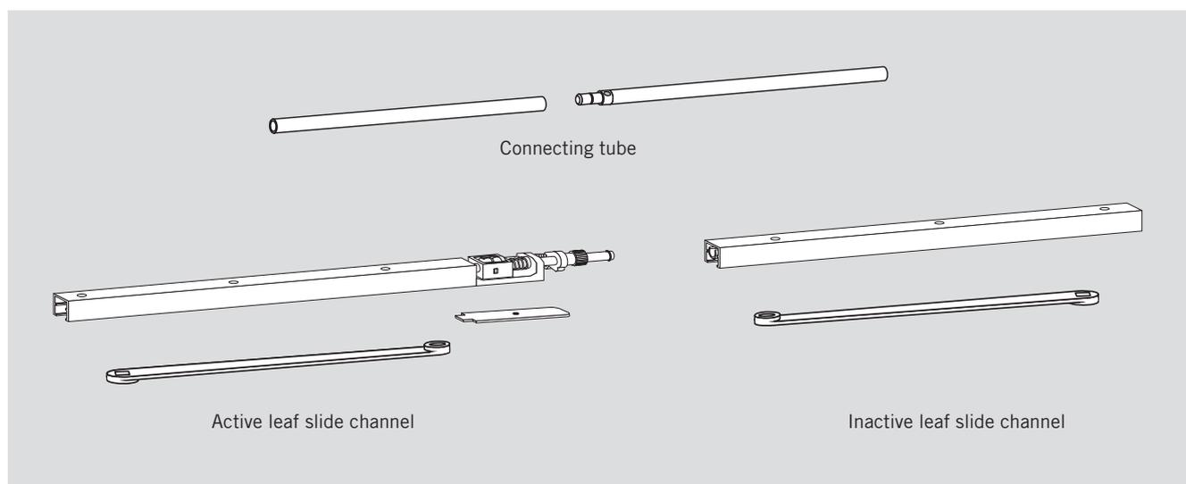
A G 96 GSR slide channel door co-ordinator encompasses an active leaf and an inactive leaf slide channel with cushioned limit stay, a connecting tube, a cover for the co-ordinator mechanism on the active leaf slide channel, and two arms.
