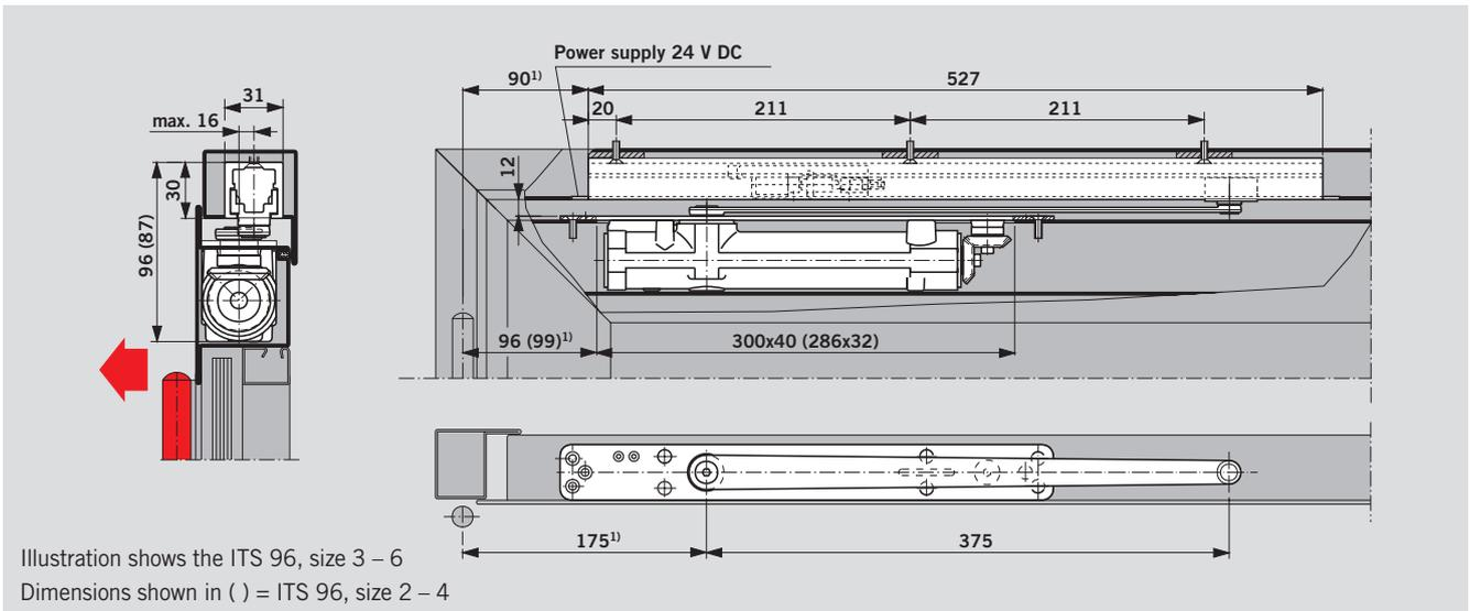
ITS 96 door closer with DORMA G 96 EMF slide channel assembly in an **aluminium framed door**.
