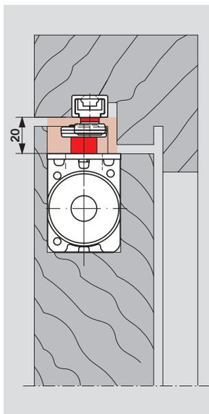
Hollow steel door with steel frame, over-rebated, clearance 12 mm, with ITS 96 EN 3-6, 4 mm extended spindle and slide channel G 96 EMF K8.
