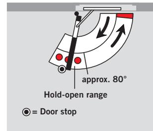
The slide channel assembly enables the door to be held open securely at a pre-selected position without fall-back. The hold-open point can be adjusted within an opening angle of approx. 80° and 120°.
