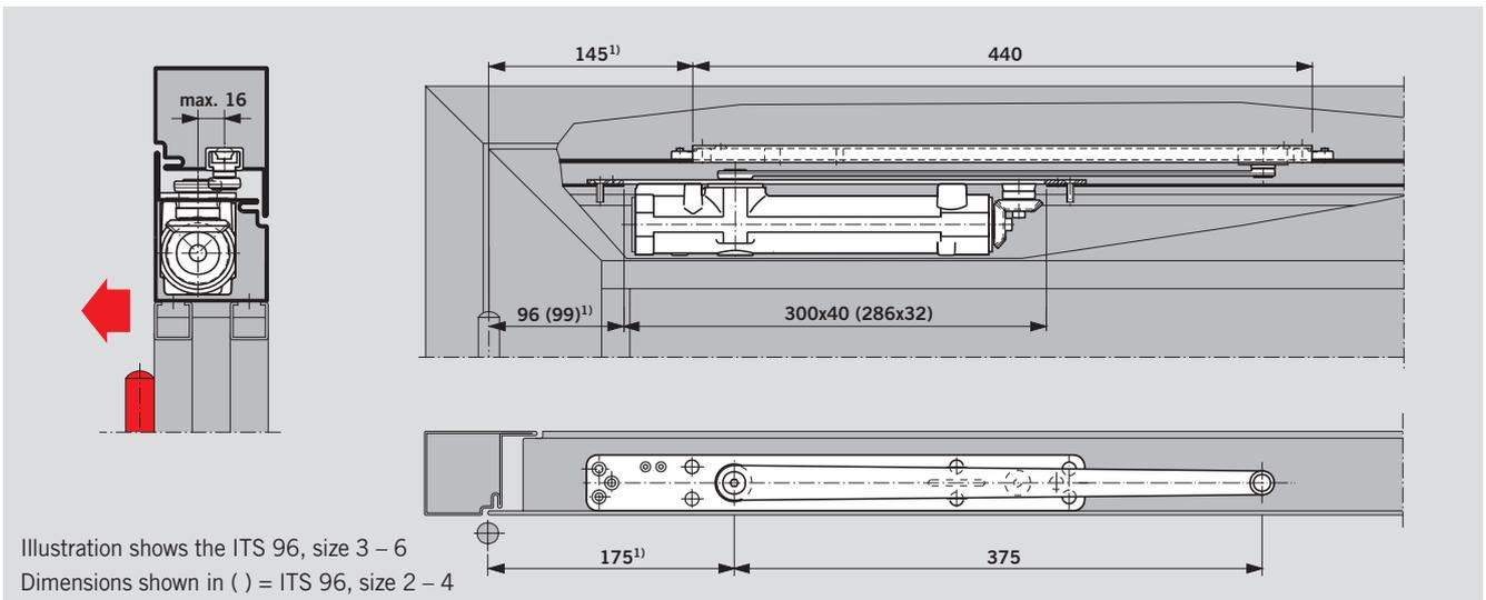
ITS 96 door closer with DORMA G 96 N20 slide channel in an **aluminium framed door**. Example: Anticlockwise-closing (ISO 6) door; mirror image applies to clockwise-closing (ISO 5) doors. <sup>1)</sup> Add 25 mm for aluminium profile frames with corner-angle reinforcement.
