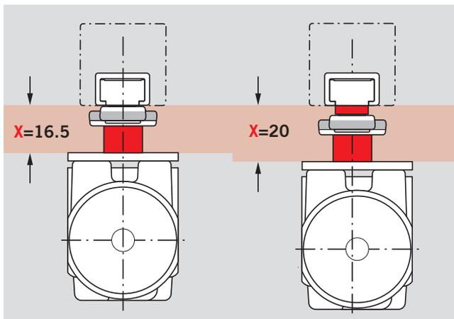
Timber door, flush-closing, clearance 8.5 mm, with ITS 96/ITS 96 FL EN 3-6 and slide channel G 96 N20 K8.
