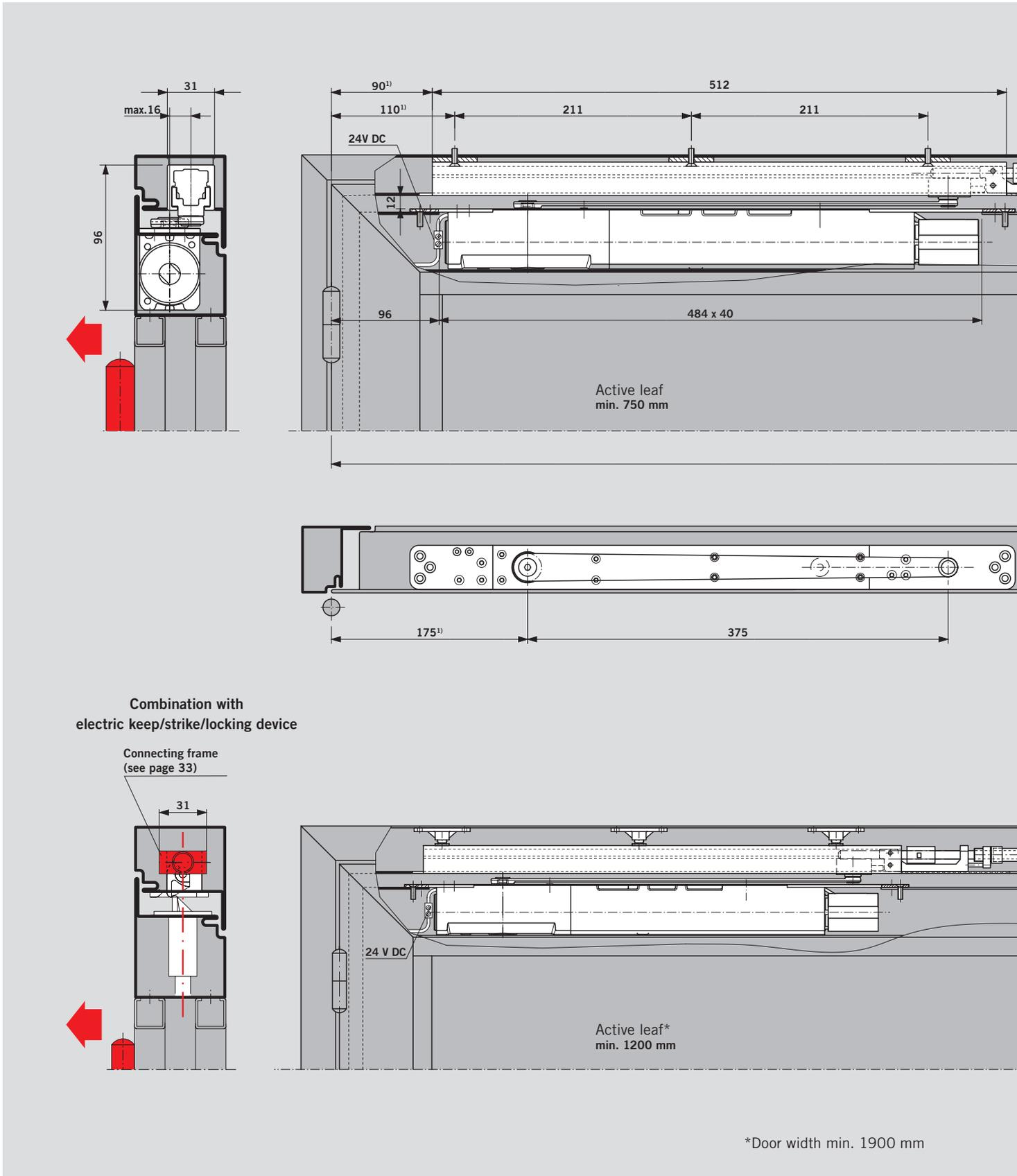
ITS 96 FL door closer at the active leaf and ITS 96 door closer at the inactive leaf with DORMA G 96 GSR slide channel.
