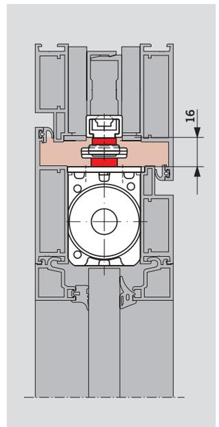
Timber door with solid frame, double-rebated, clearance 20 mm, with ITS 96/ITS 96 FL EN 3-6, 8 mm extended spindle and slide channel G 96 N20 K12.
