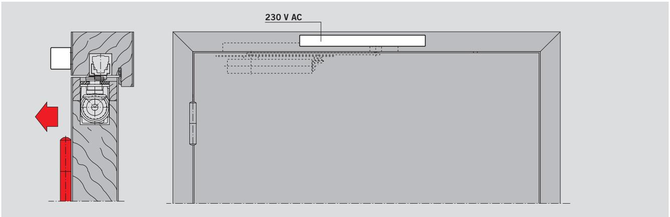
RMZ frame-mounted smoke detector on the pull side connected to an ITS 96 EMF.
