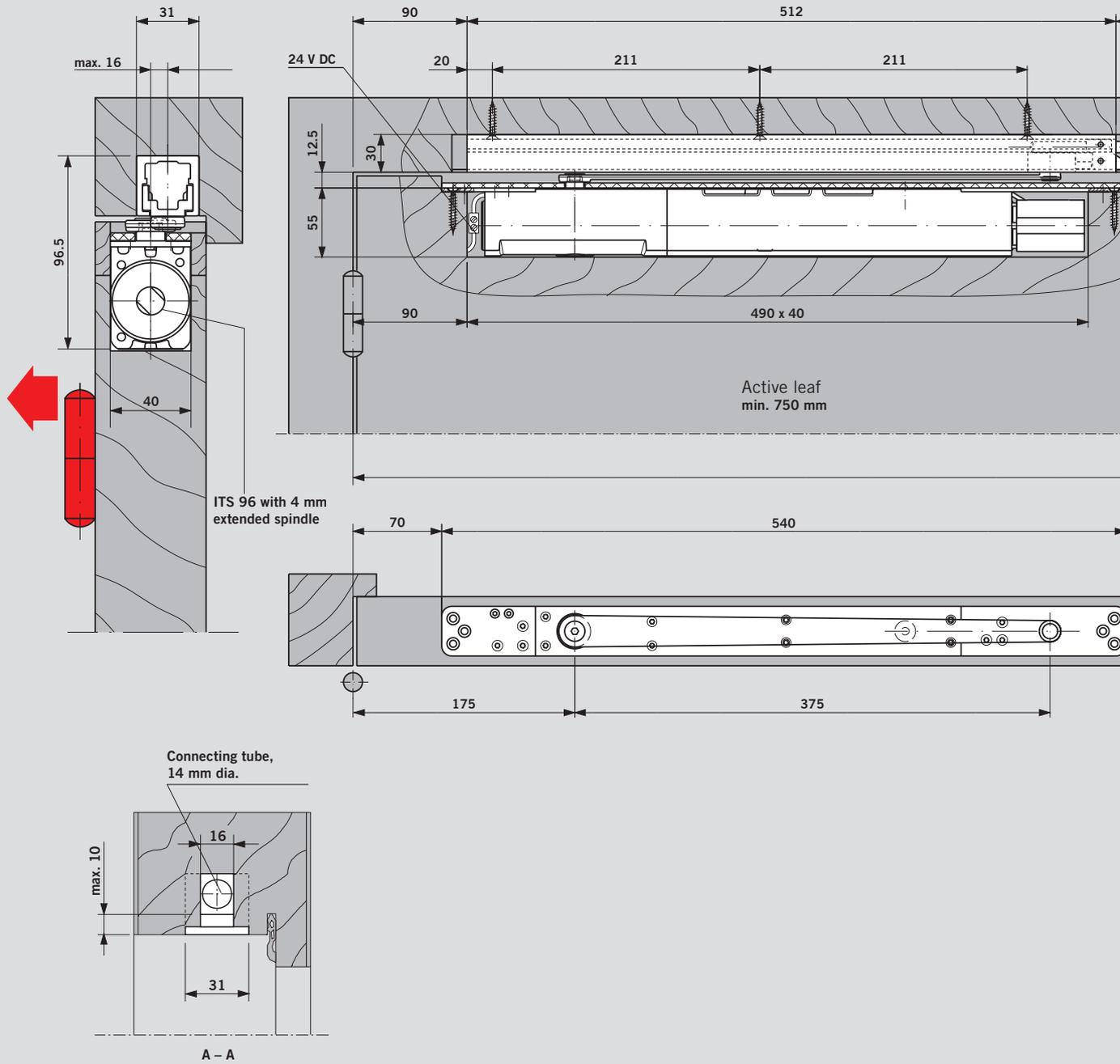
ITS 96 FL door closer at the active leaf and ITS 96 door closer at the inactive leaf with DORMA G 96 GSR slide channel.
