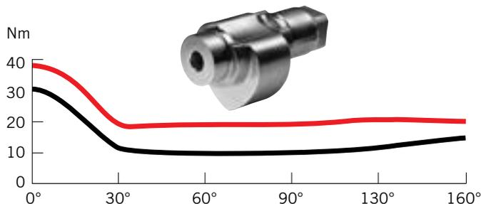
The heart-shaped cam and linear drive mechanism of the TS 97 ensure that the resistance encountered decreases almost instantly with the door opening action – so even children, the elderly and people with disabilities have no problem in passing through.
