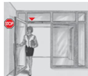
The **mechanical hold-open device** enables doors to be held without fallback at an opening angle up to approx. 120°. The hold-open device is suitable for both LH and RH doors and is designed for retrofitting into the slide channel.
