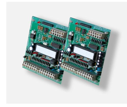
WIEEX2 receiver and transmitter modules are designed to extend the standard 500 ft (152 m) Wiegand cable distance maximum up to 4000 ft (1220 m) using proprietary RS485 communication between them.
