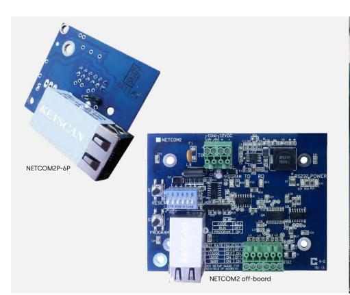
Keyscan NETCOM TCP/IP communication modules are a fast and easy way to connect your Keyscan Access Control system to your LAN/WAN network.
