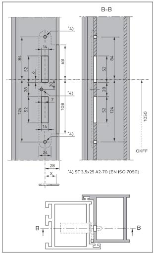
Fig. 11 Cut-outs and pre-drilled holes in door frame
