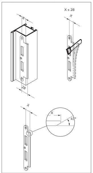
Fig. 19 Dimensions of the adjustments
