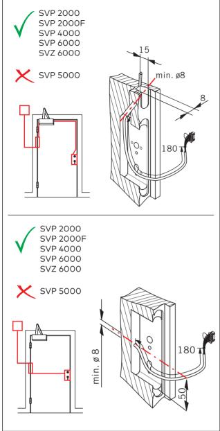
Fig. 14 Recesses and pre-drilled holes in the door leaf for wiring
