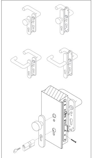
Fig. 25 Mount door handle and locking cylinder
