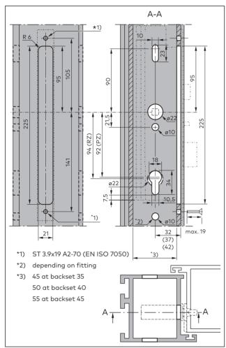
Fig. 10 Cut-outs and pre-drilled holes in door leaf
