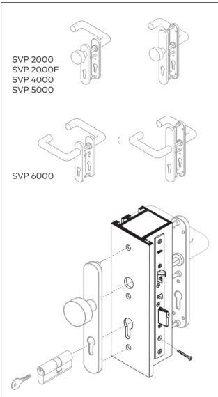
Fig. 18 Mount door handle and locking cylinder
