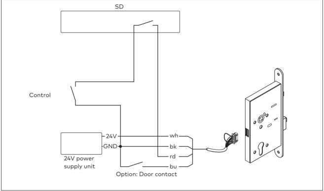
Fig. 31 Wiring of smoke detectors with a SVP 2000/SVP 2000F
