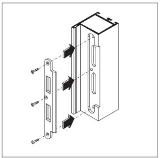
Fig. 20 Mount striking plate
