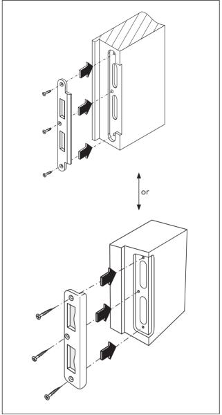
Fig. 27 Mount striking plate
