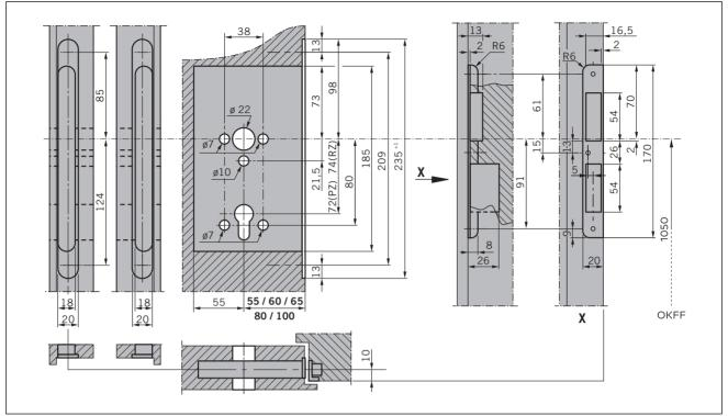
Fig. 12 Cut-outs and pre-drilled holes in the door leaf and door frame with an angled striking plate
