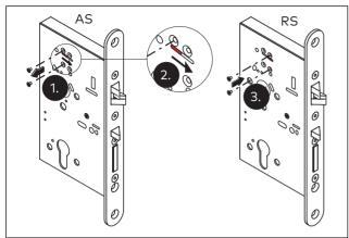
Fig. 21 Change fail secure to fail safe operating current
