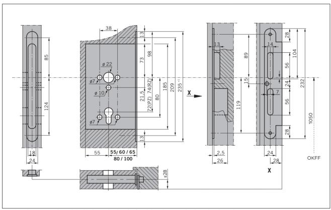
Fig. 13 Cut-outs and pre-drilled holes in the door leaf and door frame with a lipped striking plate
