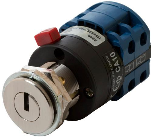
High Security 2pole, 2 position spring return changeover keyswitch with electrically isolated contacts (no links between terminals).
