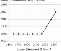
Subject to the diameter the installation height of the sensor increases in order to monitor the complete space
