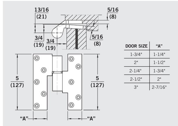
**No. 75140** — 3/4" offset brass top pivot for lead-lined doors 1-3/4" thick.
