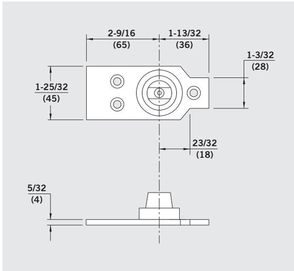
**No. 7471K** — Standard floor bearing with thrust roller bearing for doors weighing up to 440 lb. Can also be used on fire doors rated up to 3 hours. Includes cover cap. Mounts directly to floor. For use with No. 75323, 75343, 7421, 7422 and 15323 bottom arms. Available with integral spindle extensions as shown in the adjacent chart.
