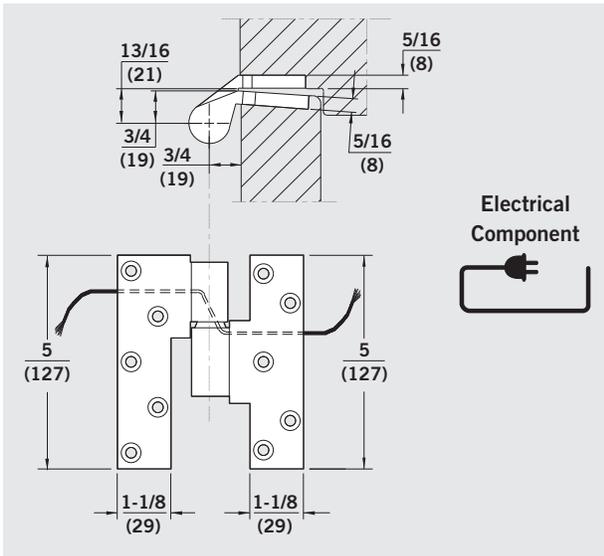
**No. 75200** — Electrified intermediate pivot for power transfer. Available as an eight-wire design using #28 AWG, rated for 24 V maximum. Pairs of wires connected together provide 2 A maximum. Multiple pairs provide greater amperage ratings, i.e. two pairs in a circuit provide 4 A maximum and four pairs provide 8 A maximum. Pivot is non-load bearing and has non-separable pivot leaves.
