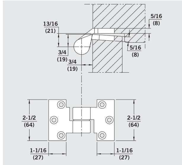
**No. 75210** — 3/4" offset light-duty brass intermediate pivot. Non-load bearing, for door alignment only.
