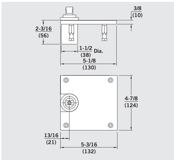
**No. 7471HD** — Heavy-duty floor bearing for center hung doors weighing up to 1000 lb and offset hung doors weighing up to 800 lb. Can also be used on fire doors rated up to 3 hours. For use with No. 7421, 75323, 75343 and 15323 bottom arms. Interchangeable spindles provide for bottom door clearances of 3/8" to 1-3/4". Includes cover plate. Bearing is mortised into floor. Interchangeable spindles and associated bottom door clearances shown in the adjacent chart.
