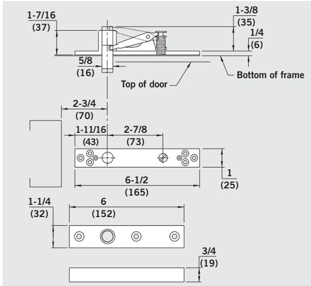
**HD8062** — Heavy-duty walking beam top pivot with frame portion and cover plate. Door portion consists of a needle bearing pressed into a 3/4" thick aluminum block. Adjustable to obtain a 1/8"–3/8" clearance between the door and frame. Required when using overhead stops/holders.
