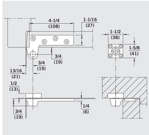
**No. 75120/102** — Standard mortised door portion with a pivot block containing a needle bearing mortised into the overhead condition above. This pivot is ideal for conditions when the door is inset from the frame face, or the ceiling is directly above the door.
