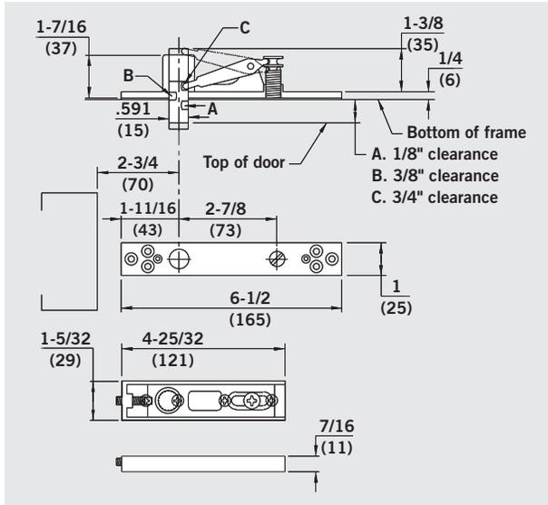
**No. 8062** — Walking beam top pivot with cover plate. Lateral adjustment assures the door is plumb. Accommodates top door clearances of 1/8", 3/8", or 3/4". Optional extended pin available for clearances of 3/4", 1", or 1-5/16". Not recommended for use with overhead stops/holders. Use HD8062.
