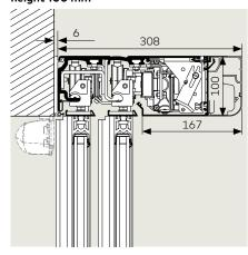
Schematic illustration of a door cross-section: wall mounted, drive height 150 mm
