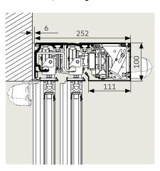
Schematic illustration of door cross-section: wall mounted, sensor casing, drive height 100 mm
