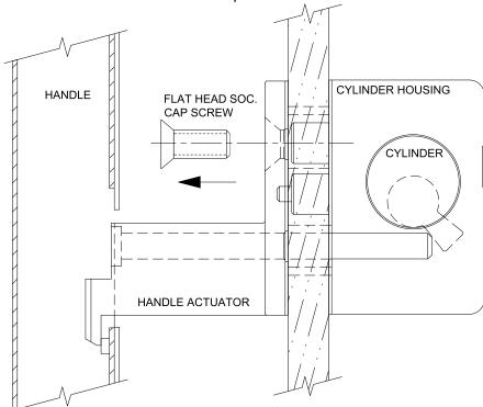
3. Pull handle away from glass. Remove handle actuator from handle.
