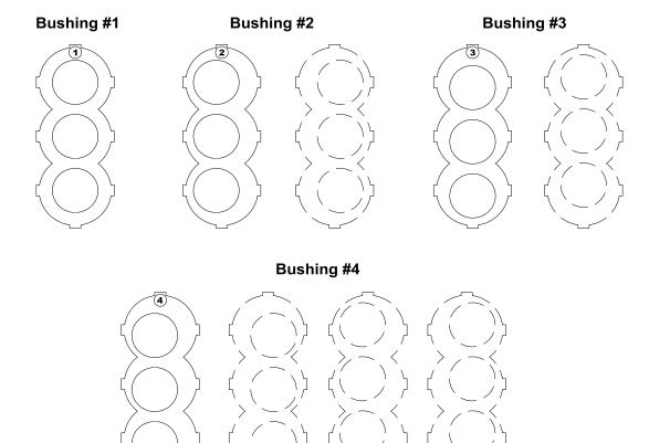
Use Bushing #4 when the "Hole Centers" and the 4 1/8" dimension from door's edge are both off 1/16" in either direction.
