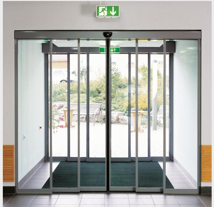
The TST FLEX Green telescopic sliding door is based on the same profile system as the ST FLEX Green sliding doors and is also an energy-saving sliding door specially designed for external building closure. The profiles have improved thermal separation and the thermal transmittance coefficients UD are proven by test certificates. Due to the slim profile elevations, this door type can be combined very well with the other door systems from the FLEX family.
