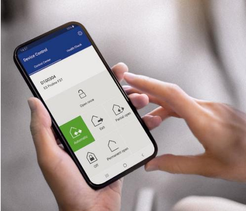
The dormakaba Door Pilot app allows automatic doors to be easily controlled from a smartphone. Operators from the ES PROLINE series can be equipped with the Door Pilot interface as an option. The app is available in iOS and Android versions and can be obtained from the respective app store.
