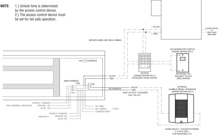
Reset and Override Wiring for Double Doors Diagram reflects status with power on
