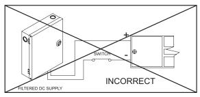
Fig. 2 - Power Connections
