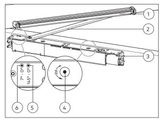
Fig. 1 TS 97 FL XEA in DIN-L mounting on the door leaf
