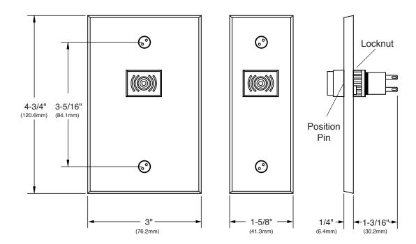
**Voltage:** 10 to 26VDC **Current Consumption:**  $\leq$  20mA
