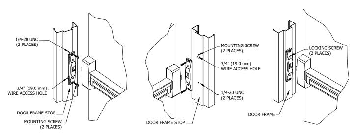
NOTE: Wire access hole locations are relative to the exit device orientation. NOTE: Not to scale. Specifications are subject to change without notice.
