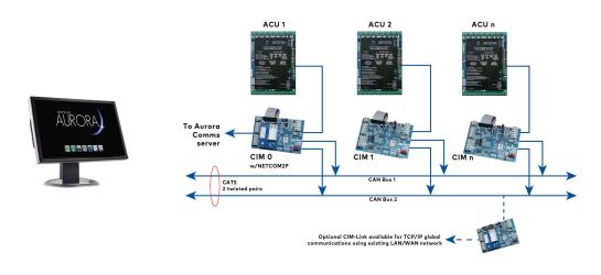
PC / ACU Bit Rate 9600 or 19,200 57,500 115,200 CAN Bus 1 & 2 CAT 5 Distance\* 3280 ft (1000m) 984.25 ft (300m) 262.46 ft (80m) RS-232 Serial Distance 49.2 ft (15m) 26.2 ft (8m) 9.84 ft (3 m)
