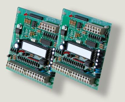
WIEEX2 receiver and transmitter modules are designed to extend the standard 500 ft (152 m) Wiegand cable distance maximum up to 4000 ft (1220 m) using proprietary RS485 communication between them.
