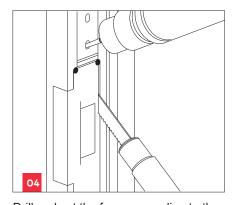
Drill and cut the frame according to the template.
