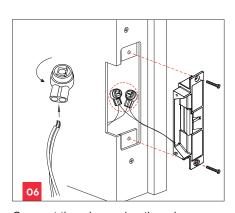
Connect the wires using the crimp connectors, and then test the strike.
