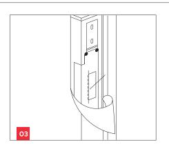
Mount the supplied template and align to the marked line.
