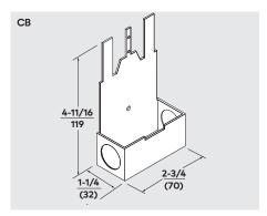
**CB** — UL approved conduit box accessory to provide surface wiring of 120 VAC power to ED900.
