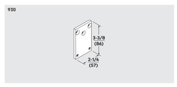
930 — For mounting arm shoe in top jamb drop application when top door rail is less than 4-5/8" (2" minimum required).
