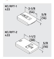
KC/RFT-1 433 (Single Frequency), KC/RFT-2 433 (Dual Frequency) — Similar to HH/RFT-1 433 or HH/RFT-2 433, but more compact. Must be used with RFR 433 receiver. KC/RFT-2 433 requires one RFR 433 per frequency. The small size permits the use as a key chain or in cases where the hand held transmitter is too large. Powered by a watch battery.
