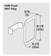
UMB Flush MNT Ring — Black ABS flush mount ring and metal mounting bracket. The ring is designed to cover the gap between the mounting box and the switch plate cutout in the wall for a nice clean look.
