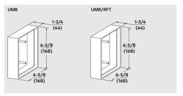
${f UMB}-{f Black}$  ABS universal replacement mounting box for WS-1 type switches.
