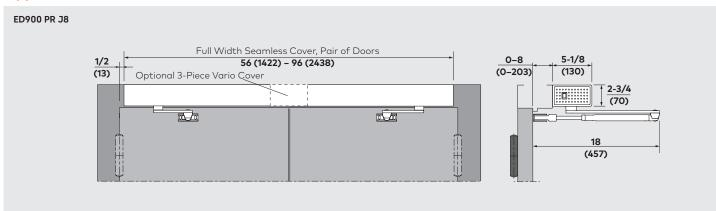
**Note**: Refer to the included bumper/stop to limit door travel to a maximum 110° to prevent possible damage to the ED900 arm. Where this is not practical, the ED900 J × Drop Mount with a surface door stop is recommended.
