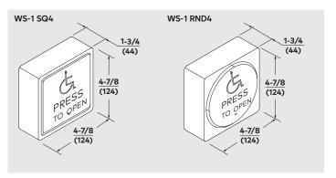
**WS-1 SQ4** — Tamper-resistant 4-1/2"  $\times$  4-1/2" wall plate with a normally open switch. Includes a heavy duty injection molded black ABS mounting box. Satin stainless steel wall plate with blue engraving. Wall plate displays the accessibility symbol and "PRESS TO OPEN." Fits a standard 4"  $\times$  4" electrical box. Must be hard wired. Flush design allows the optimum in weather resistance, in surface, or recessed applications.
