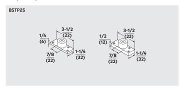
BSTP25 (1/4" thick base plate)/BSTP50 (1/2" thick base plate)—
