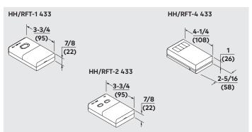
HH/RFT-1 433 (Single Frequency), HH/RFT-2 433 (Dual Frequency), HH/RFT-4 433 (Quad Frequency) — Compact, portable, 433 MHz switches. Must be used with RFR 433 receiver. Maximum range is approximately 50 ft (depending on conditions). Powered by 9 VDC battery.
