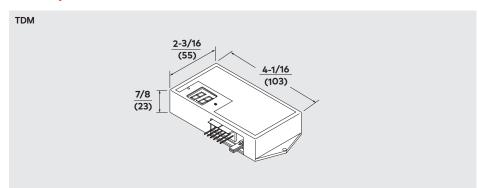
${\sf TDM}$  — Advanced time delay module, allowing the installer to use only one time delay for any automatic door operation, on electrically or magnetically locked doors. TDM is required for vestibule sequencing and simultaneous triggering of (2) ED900 operators.
