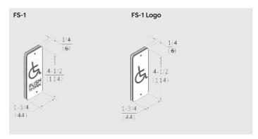
**FS-1** — 1-3/4"  $\times$  4-1/2" frame plate with a normally open switch. Satin stainless steel frame plate with blue engraving. Frame plate displays the accessibility symbol and "PRESS TO OPEN." Fits a minimum 1-3/4"  $\times$  4" frame section. Must be hard wired.
