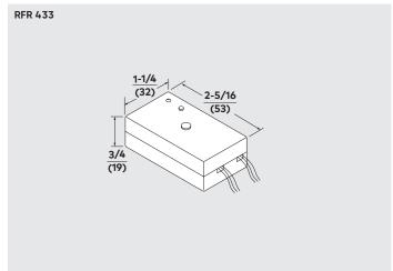
**RFR 433** — Radio frequency receiver, 433 MHz. Required for use with all DORMA transmitter switches. Powered from the onboard power supply of the ED900. Ideal for applications with range and signal strength problems.
