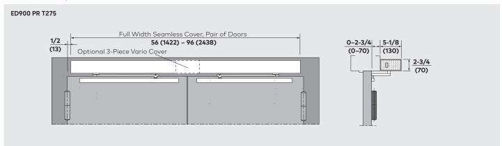
**Note**: Refer to the included bumper/stop to limit door travel to a maximum 110° to prevent possible damage to the ED900 arm. Where this is not practical, the ED900 J × Drop Mount with a surface door stop is recommended.
