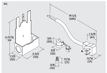
**PC** — Eliminates need for hard wiring. Permits ED900 to plug directly into 120 VAC/60 Hz receptacle. Cord measures 15" from end cap to center of plug.
