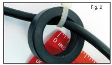
1. Insert the mini USB end of the cable into ferrite ring with 8.5" protruding (Fig.1).
