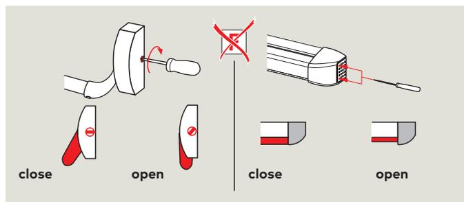
The dogging device serves to hold the latch in its retracted position so the door is freely accessible.
