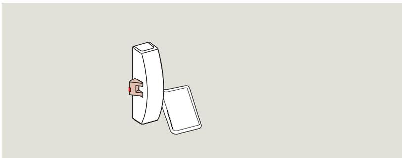
The security anti-thrust latch prevents the latch from being pushed back by unauthorised means when it is in the closed position.
