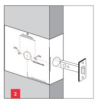
Drill holes in accordance with the template.
