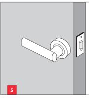
5. Install furniture to the door do not tighten screws with excessive tension on power driver as this may damage screws and void warranty. Fit and align round outer rose.
