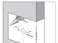
1. Position template and mark out drilling centres. Important also refer to lock/latch manufacturer's template prior to drilling. This template applies to bolt through fix lock/latch with a 60mm backset.
