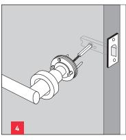
4. Insert spindle and spring supplied with levers to both sides of the door, as shown. Determine the correct screw length to suit the door thickness then cut screws.
