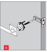
4. Insert spindle and spring supplied with levers to both sides of the door, as shown.
