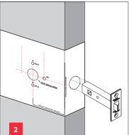
2. Drill holes in accordance with the template.
