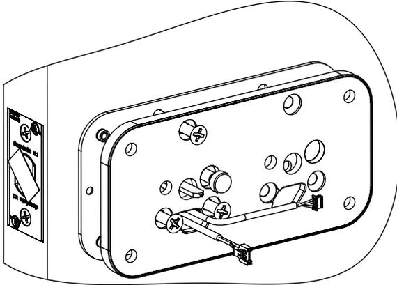
1. Harness shall be pulled gently through inside trim's backplate to accumulate all excess cables within the inside trim.
