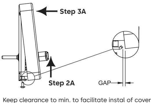
**Step 2B:** Engage cover's tab in back plate's hook. Lift cover as required.
