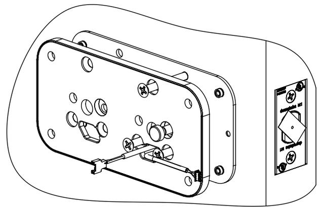
1. Harness shall be pulled gently through inside trim's backplate to accumulate all excess cables within the inside trim.
