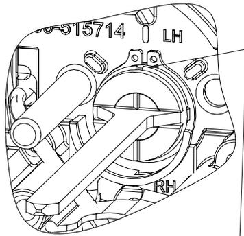
Tail piece shall be "snap" in place with wire ring opening rotated at 12 o'clock
