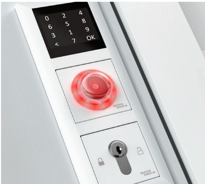
The SCU-UP with emergency button is always used with a key switch (e.g. analogue ST 55 key switch). Together with an electrical locking device, the SCU-UP fulfils the requirements of EN 13637 and EltVTR (German directive for electrical locking systems on escape route doors).
