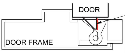
Ensure a minimum 1mm gap between the latch and the front face of the release plate to avoid pre-load on strike.
