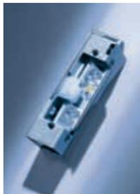
Electric strike with adjustable latch, suitable for over-rebated and flush-closing doors, non-handed. 24 V DC, 130 mA
