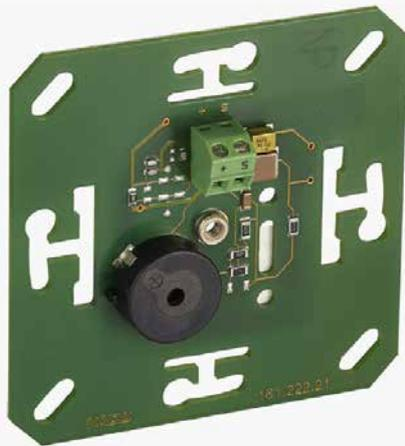
*The Kaba registration unit 90 00 provides freedom of design: it can be built into customised or standard housings. The component fits into various European standard covers.*
