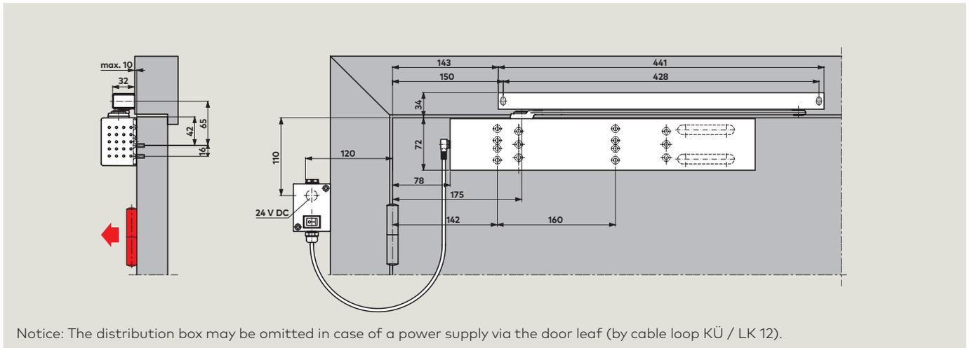
Door closer **TS 99 FL in standard application** (door leaf fixing)
