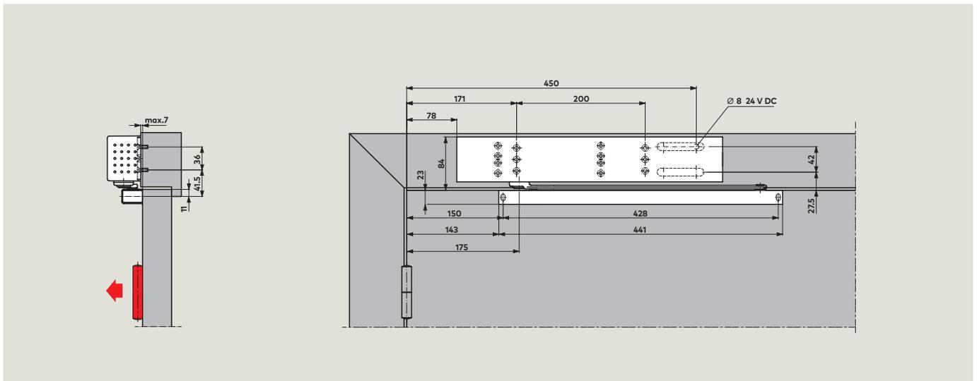
Door closer **TS 99 FL in frame mounted** (transom fixing)
