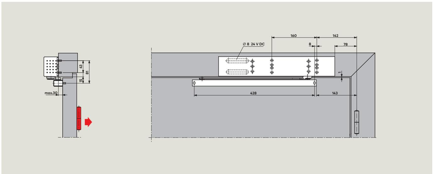
Door closer **TS 99 FL in frame mounted on push side** (transom fixing)
