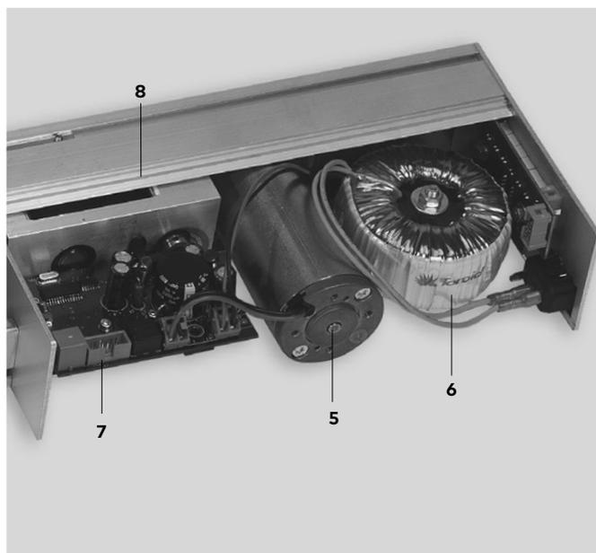
The prefabricated drive unit consists of all required electrical components and is tested individually thus facilitating the assembly and maintenance of the operator.
