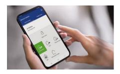
The drives of the ES PROLINE series are optionally equipped with the Door Pilot Interface. Via the Door Pilot app, various status messages of the drive can be read out easily using a smartphone and functions can be controlled. Another service advantage of the new drive system.
