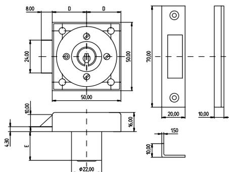
E = Installation depth in mm
