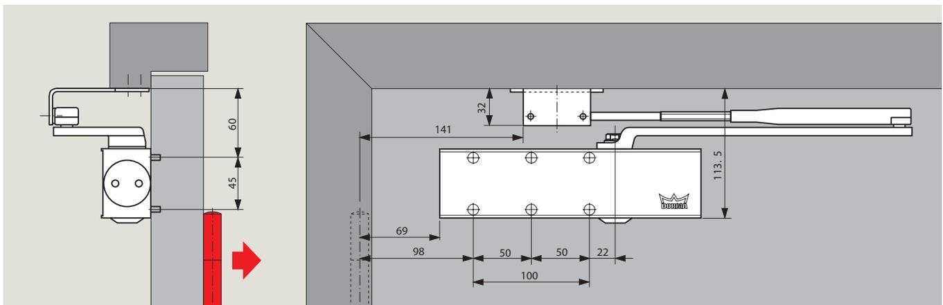
With transom-fixed closers, the backcheck comes in later at between 85° and 90°, depending on the door thickness and projection of the hinge used.
