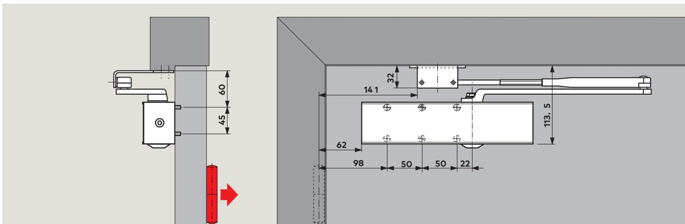
With parallel arm application, the backcheck comes in later at between 85° and 90°, depending on the door thickness and projection of
