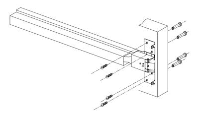
3) INSTALL END CAP MOUNTING BRACKET USING MOUNTING SCREW.
