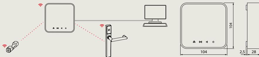
The dormakaba wireless gateway 90 40 communicates with the access components by radio frequency and is connected to the access control system through an ethernet cable.
