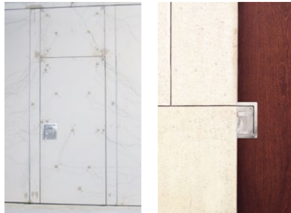
In order to ascertain the fire resistance class, a wall comprising Variflex EI 30 panels with an integrated passdoor was directly subjected to fire for longer than half an hour in a test lab.
