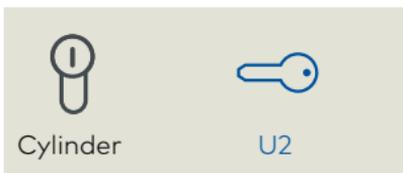
Changing key U2 is used: Pin combination is modified in the cylinder
