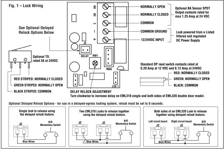
6. To Ensure Instant Release All switching devices must be wired in between the DC power source and the positive terminal of the lock in Fig. 3. Switching the negative power supply line will not allow the lock to release immediately.
