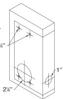
A-2 Mortise door edge for latch unit faceplate (c) ½" (3 mm) deep to dimensions shown. Insert latch unit (a) into the 1" (25 mm) hole, making certain that the latch bolt bevel faces direction of closing door.
