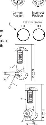
Insert the supplied tailpiece (e) vertically into the outside lever/knob (b) as shown. Make certain that you rotate the tailpiece so it will align with the interchangeable core. For screw cap type cylinders (Schlage) (g), the tailpiece must be assembled to the cylinder first with the tailpiece vertically as shown. Insert the core into the outside lever/knob.
