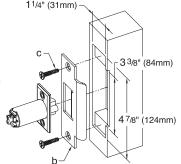
Caution: Check the operation of the latch by making sure that the deadlatch (a) stops against the strike (b) as shown and does not slide into the strike opening when the door is closed. If that situation occurs, then a total lockout may occur. This will void our warranty of the complete lock mechanism. If necessary, correct the door over-travel by using the rubber bumpers as described in Section N (Installing Rubber Bumpers).
