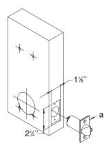
**A-3** Secure the latch to the door using two ¾" (19 mm) combination screws (b) supplied. Latch unit faceplate must be flush with door (c).
