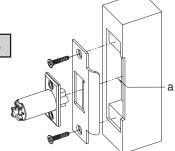
M-2 Mortise doorframe for strike <sup>3</sup>/<sub>32</sub>" (3 mm) deep minimum to dimensions shown. Secure strike (b) to the door frame using two 1" (25 mm) combination screws (c) (supplied).
