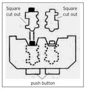
the tumblers into the lock body, they must be fitted facing the correct way as show in the illustration.
