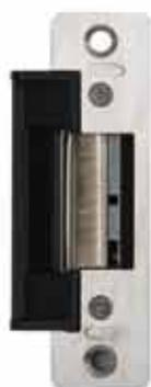
The electric strike is designed to release the door-locking mechanism when electrical power is applied. It works with mortise, rim, and cylindrical locks. Different models and sizes are available depending on the application. All models are fail-secure.
