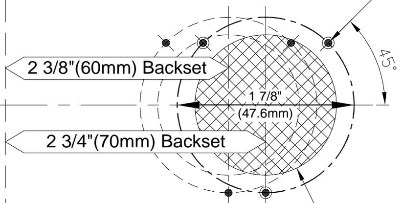
Use 1" (25mm) drill for deadbolt hole, depth is 4" (102mm) minimum
