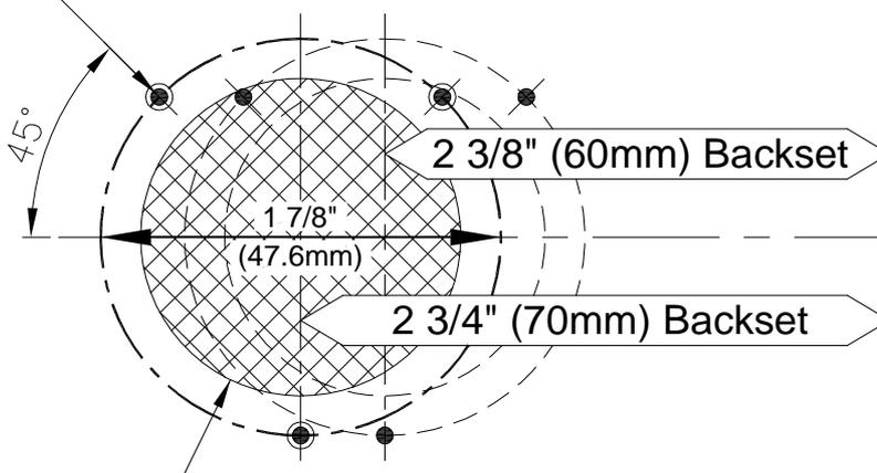
Drill  $1 \frac{1}{2}$ " (38.1mm) dia. hole and  $1 \frac{3}{16}$ " (30mm) depth.
