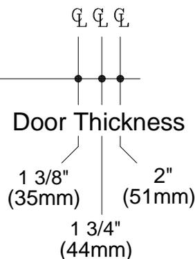
Use 1" (25mm) drill for deadbolt hole, depth is 4" (102mm) minimum
