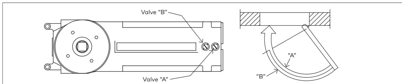
2.3.1 Valve "A" - controls closing speed from maximum opening angle to 0°.
