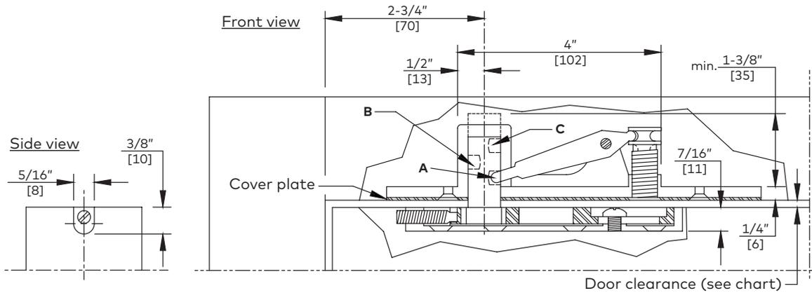
For 10-32 machine screws use No.21 drill.
