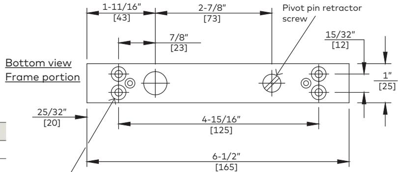
For 10-32 machine screws use No.21 drill.
