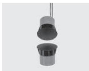
**MC-7**—Self-locking recessed mount with 1" dia. magnetic contact. Accommodates up to a 1/2" gap between the door and frame. SPDT 250 mA @ 30 V AC/DC, #22 AWG
