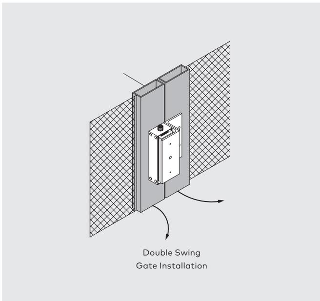
**NOTE:** For proper operation, one side of the double gate pair should be stationary. Lock may not hold correctly if both gates swing freely.
