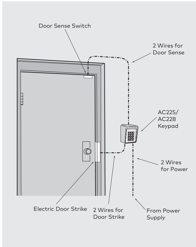
**Typical Door Installation Wiring**
