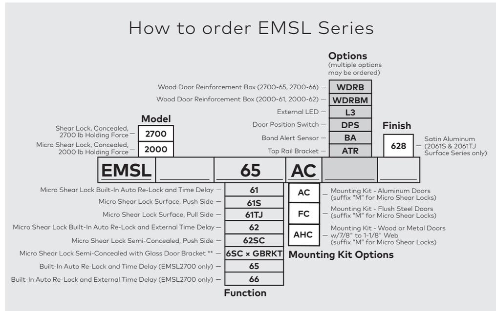
**EMSL2000-62SCGDB-KT3/4**—Semi-concealed with glass door bracket, 3/4" glass. Lock is mortised.
