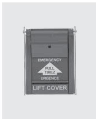
**39043 Emergency Pull Station**—Enables emergency release for electromagnetic locks. Clear polycarbonate cover lifts easily so paddle can be pulled forward, instantly releasing lock. Available in molded yellow or blue with red pull.
