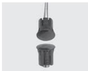
**MC-4**—Self-locking recessed mount. 3/4" dia. magnetic contact. Accommodates up to a 1/2" gap between the door and frame. SPDT 250 mA @ 30 V AC/DC, #22 AWG
