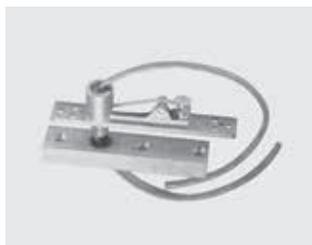
**E80622, 2 wire/E80624, 4 wire**—Electrified walking beam top pivot for power transfer. Available in a two-wire and four-wire design using #18 AWG. Both designs provide a maximum of 6 A @ 24 V. Specify number of wires required
