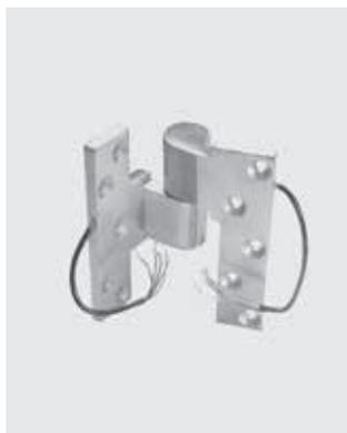
**75200**—Electrified intermediate pivot for power transfer. This eight-wire design uses #28 AWG, rated for 24 V maximum. Pairs of wires connected together provide 2 amps maximum. Multiple pairs provide greater amperage ratings, i.e. two pairs in a circuit provide 4 A maximum, and four pairs provide 8 A maximum. Pivot is non-load bearing and has non-separable pivot leaves. Specify Hand.
