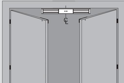
**NOTE:** A minimum distance of 1-5/8" (41.3 mm) is required without the need of a mounting accessory. Should you require a mounting accessory please see our literature or contact Customer Service.
