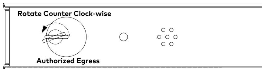
**NOTE:** The **By-pass mode** and **Re-arm mode** (orange wire) may be initiated externally from the terminal connector. (Normally open dry contact to ground.) The **Authorized Egress mode** (white wire) may be initiated externally from the terminal connector (Normally open dry contact to ground). See page 6 for additional details.
