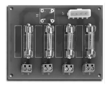
The optional FB-4 provides four (4) individually fused outputs for modular system protection. The fuse rating for each output is determined by the load current of each output. The fused voltage output is the same as the voltage input. The total current of all outputs can not exceed the power supply rating of 1.5 Amps Maximum.
